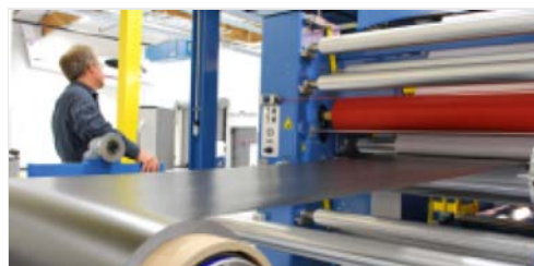
TenCate's 50-inch-wide precision uni-tape machine produces TC250, a toughed OOA epoxy prepreg system for aerospace applications.
