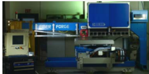
Fiberforge's Relay™ manufacturing system uses prepreg tape in an automated lay-up process to produce tailored blanks, which are thermoformed into finished parts.
