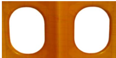
Aircraft cabin sidewall was manufactured by Diehl Aerospace GmbH using Gurit's PB1000 prepreg.
